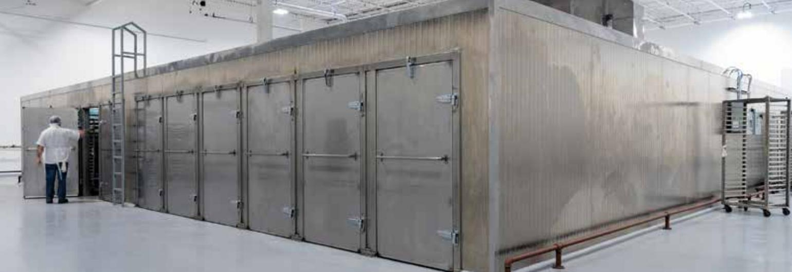
Fireking has two proofers and two retarders designed by the bakery's engineers to provide capacity during busy season and redundancy in case of downtime.
