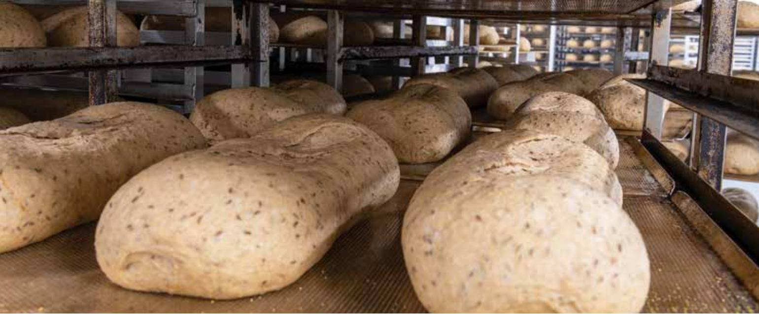
After makeup, dough retards in a custom-built cooler. Humidity prevents the dough from drying out and cracking on the surface.
